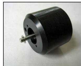
Next, screw the small metal plate onto the bottom to hold the shaft in place, using the two tiny wood screws.
