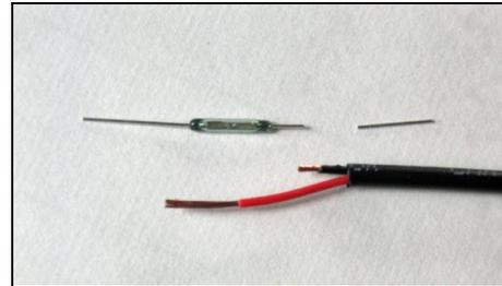
**The reed switch is inside the section of straw. HANDLE THE REED WITH CARE. Never bend the wire while holding the reed switch – it will break!**
