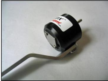
At this point, check that the reed/wire fit in the hole. CAUTION: any bending will crack the reed and break it. It needs to slide in the hole, all the way to the bottom, without effort.
